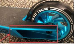
Exposed metal sections of the scooter deck. These sections are present in both the Teal/Chrome and the Gold/Black models.
