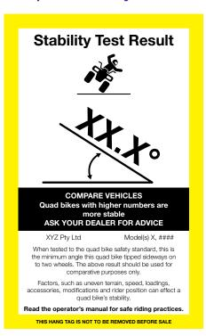
The hang tag will tell you the minimum angle at which the quad bike tipped sideways on to two wheels when it was tested by the manufacturer. Quad bikes with higher numbers are more stable.
